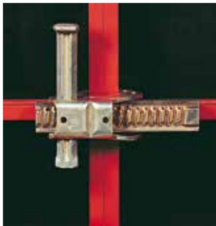
The Alignment Coupler DRS on a standard panel joint ... ... and with timber compensations up to 10 cm thick.
